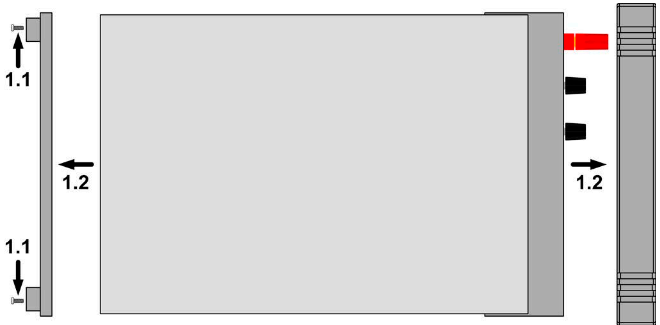
Figure 7 - Removal of the front and rear frame
